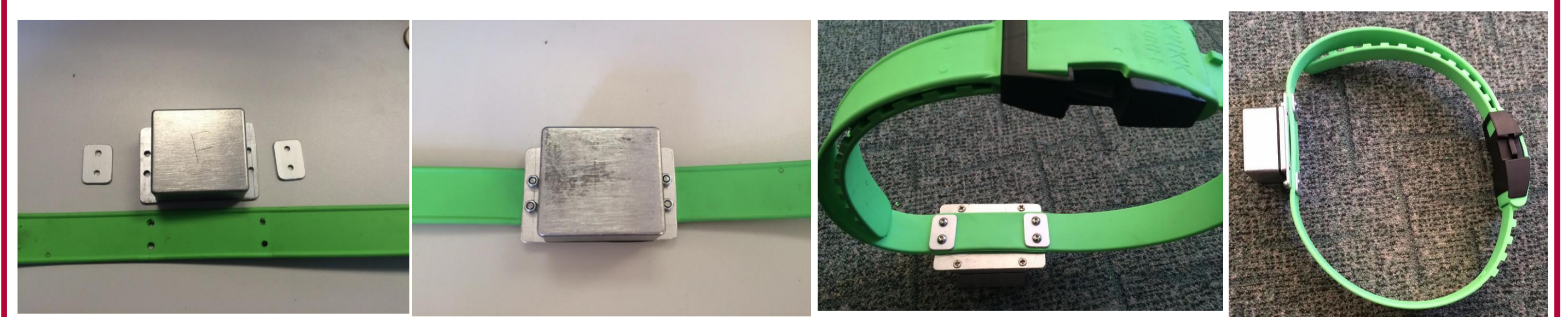
Attaching a dosimeter box to the example reindeer collar
